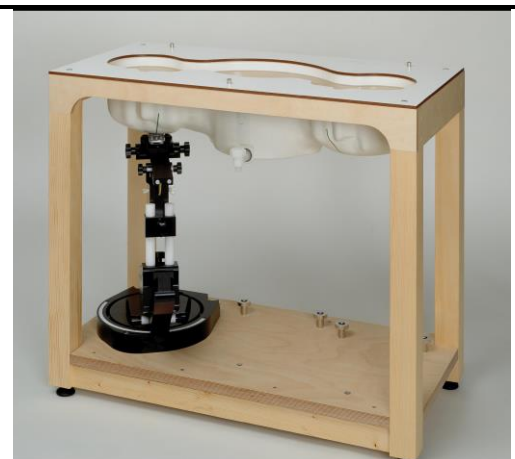
Fig. 8.7 Photo of SAM Twin Phantom
