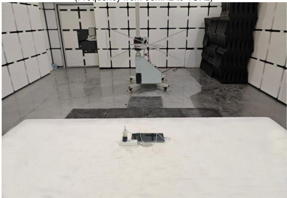
RADIATED EMISSION TEST
