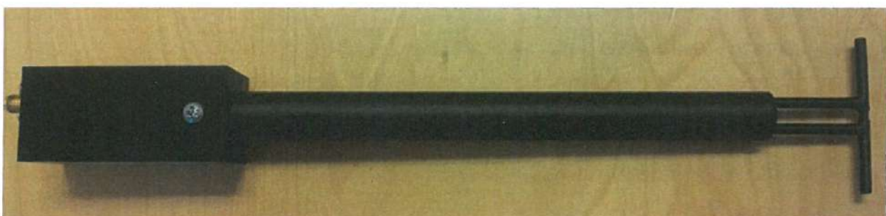
Figure 1 – MVG COMOSAR Validation Dipole
