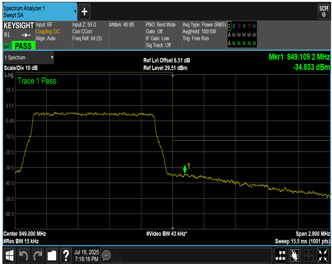
Band5 QAM16 BW=5MHz Channel=20625 RB Size=25 Position=#0
