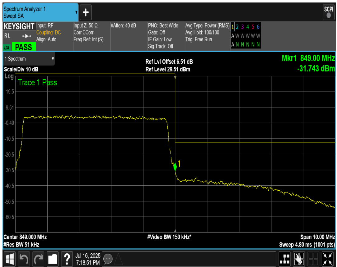
Band5 QPSK BW=1.4MHz Channel=20407 RB Size=6 Position=#0
