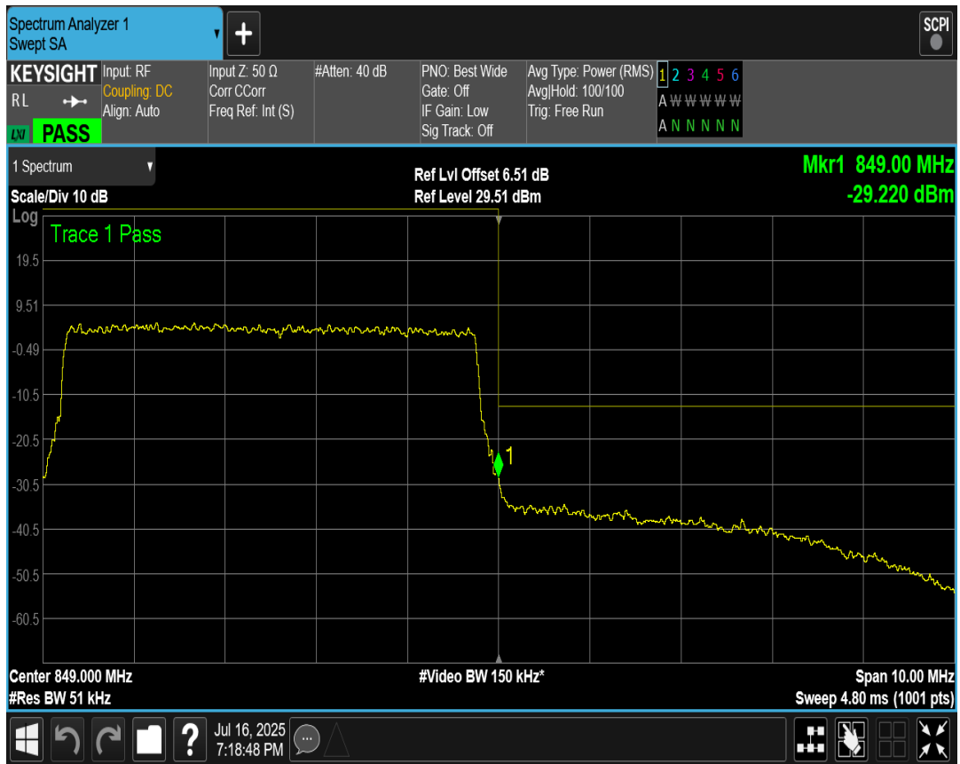
Band5 QPSK BW=3MHz Channel=20415 RB Size=15 Position=#0
