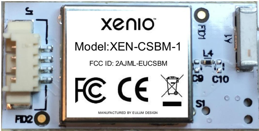
Label is applied to the RF shield. Placement is the same for all models (i.e. all models use the same RF shield).
