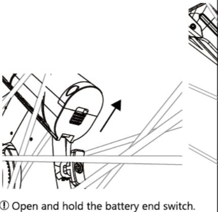
① Open and hold the battery end switch.
