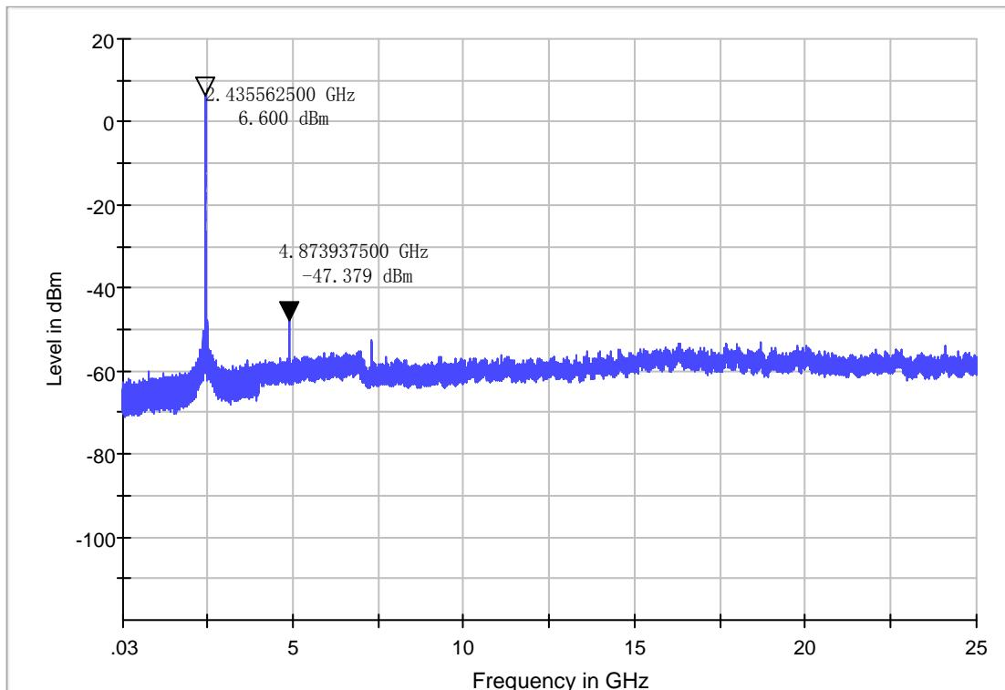
In any 100kHz bandwidth, the Conducted Spurious Emissions from 30 MHz to 25 GHz were greater than 20dB below the peak emission within the band that contains the highest level of the desired power.
