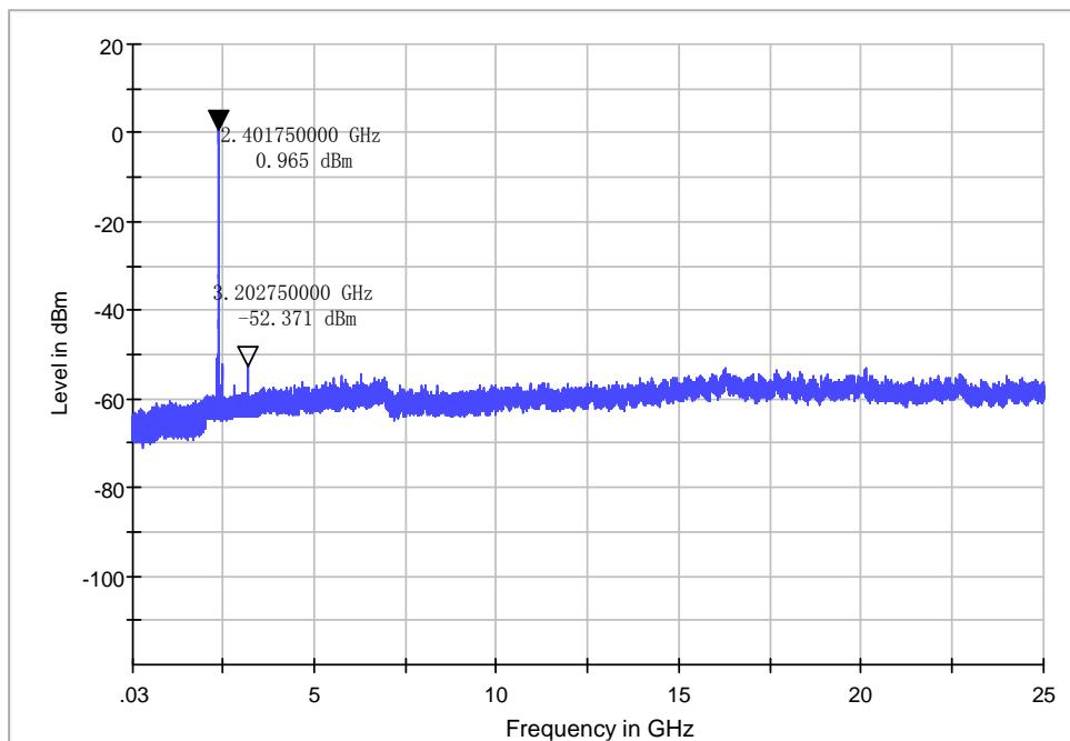
In any 100 kHz bandwidth, the Conducted Spurious Emissions from 30 MHz to 25 GHz were greater than 20dB below the peak emission within the band that contains the highest level of the desired power.
