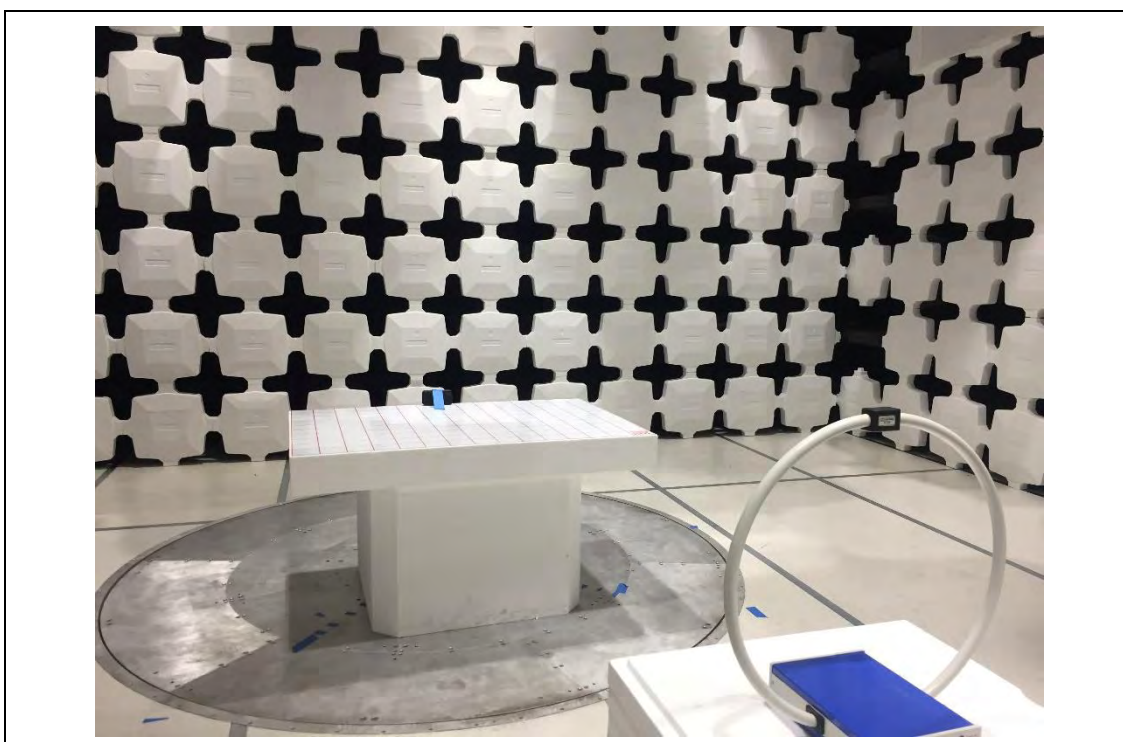
Radiated Emissions Below 30MHz setup – Front
