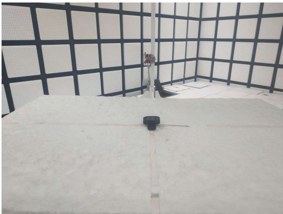
Radiated spurious emission Test Setup-2(Above 1GHz)
