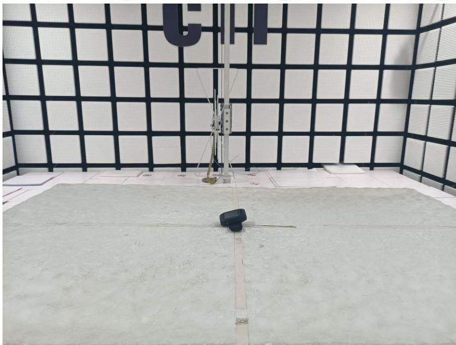
Radiated spurious emission Test Setup-1(Below 1GHz)
