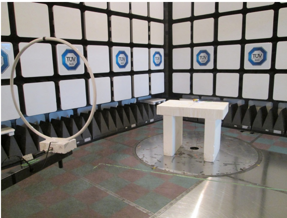
Test setup photo 1 Radiated measurements, 9 kHz – 30 MHz
