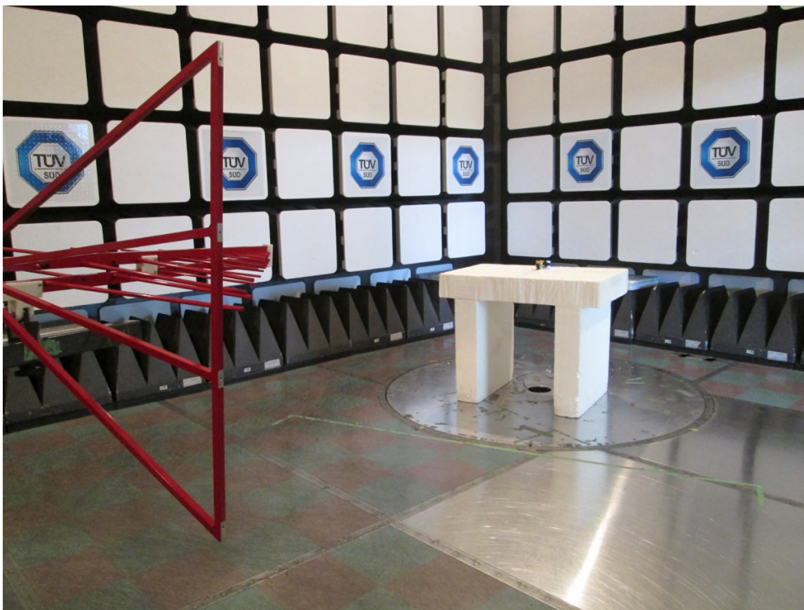
Test setup photo 2 Radiated measurements, 30 MHz – 1 GHz
