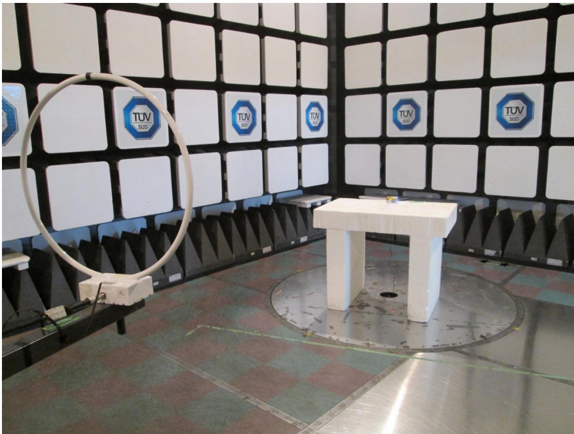
Test setup photo 1 Radiated measurements, 9 kHz – 30 MHz
