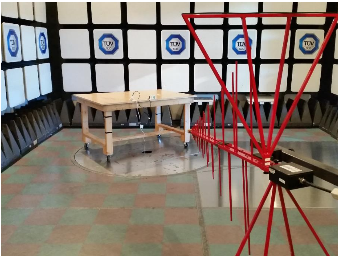
Figure 3 – Radiated Emissions Setup – Photo 2
