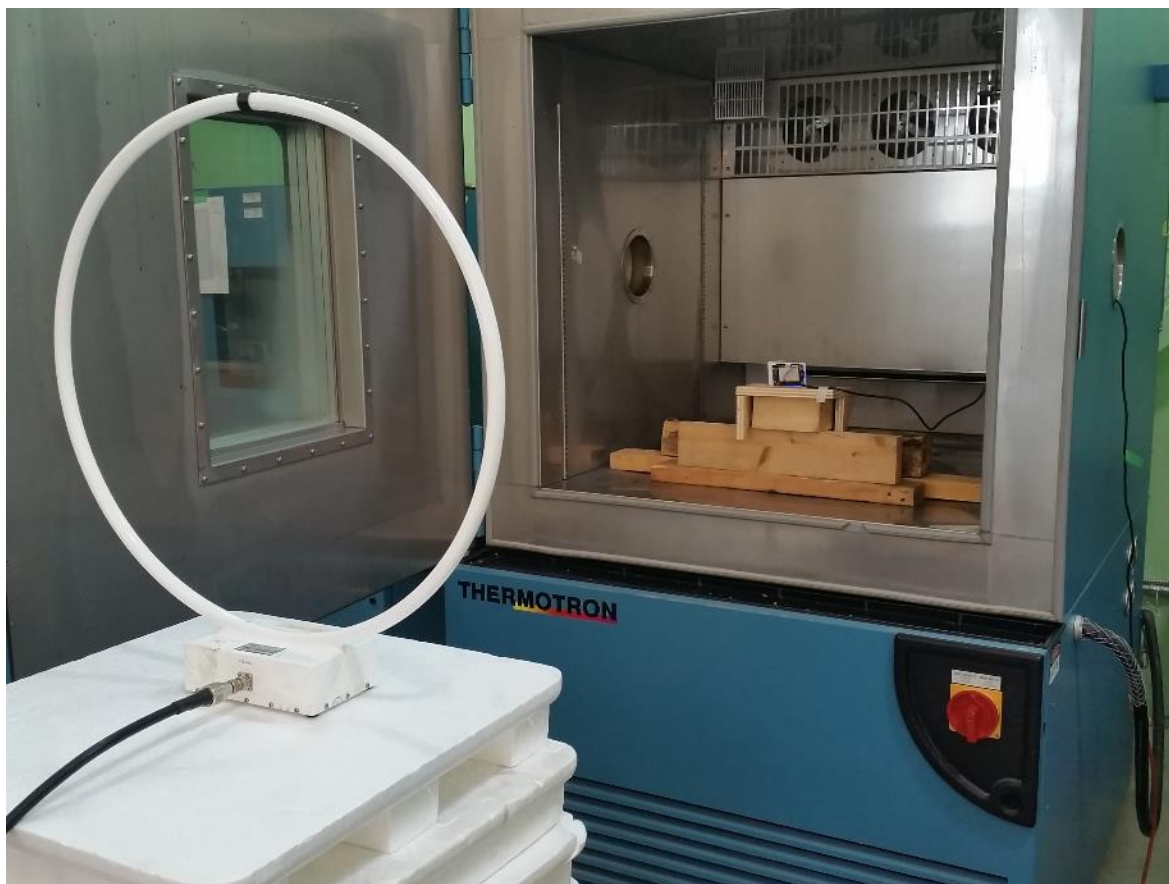
Figure 4 – Carrier Frequency Stability Setup
