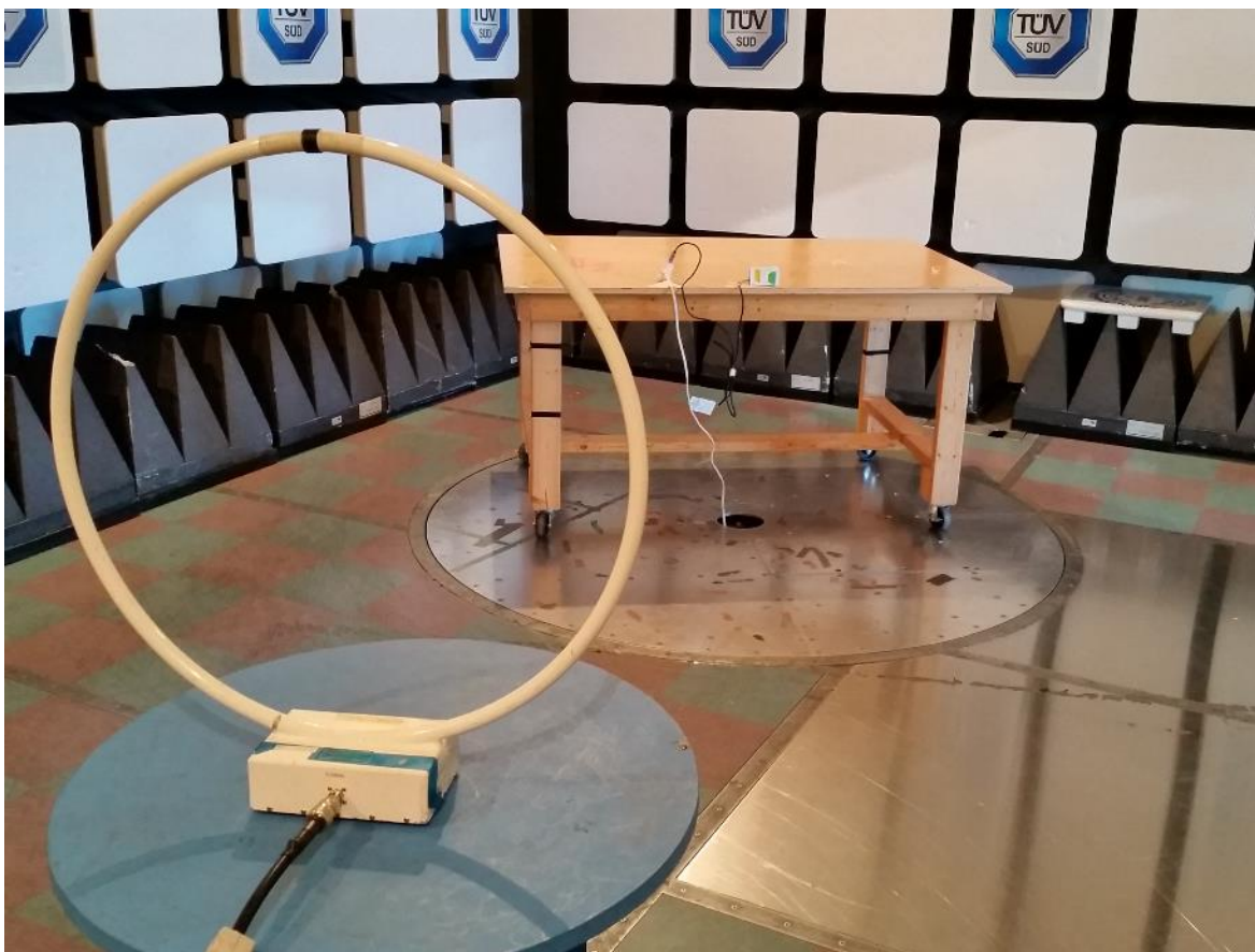
Figure 2 – Radiated Emissions Setup – Photo 1
