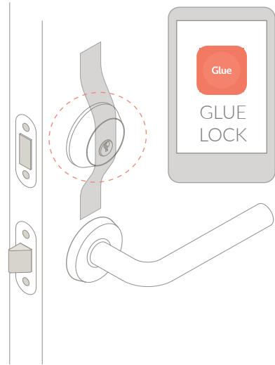
Step 1. Download the app. Secure the lock cylinder on the outside of the door with tape. This ensures it is held securely in place, whilst you fit your Glue Smart Lock.
