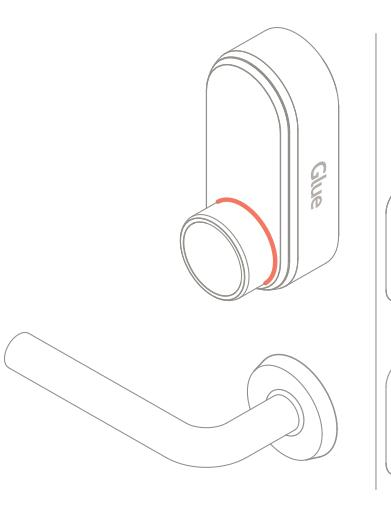
Step 10. Screw the Glue Smart Lock to the door plate. Turn the thumb turn on the Glue Smart Lock to check the latch opens and closes smoothly, if not return to Step 4.
