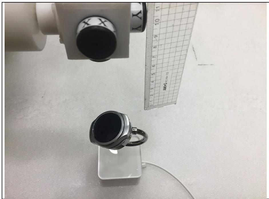
***B. B-Field Probe*****Probe Position A**
