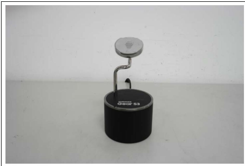
**2. Photo of Radiated Spurious Emission Test (Below 30 MHz)**
