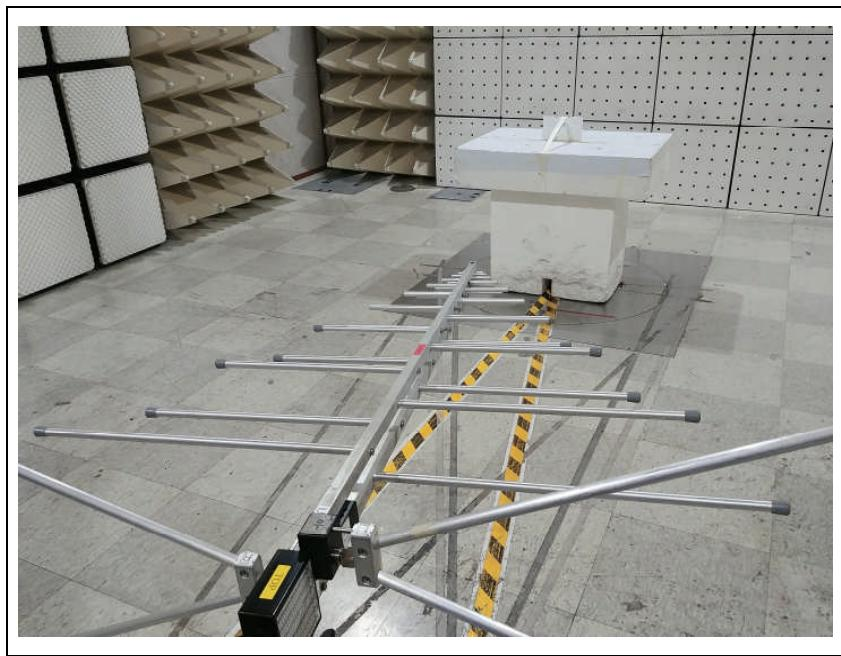
**- Photo of Radiated Spurious Emission Test (Above 1 GHz)**
