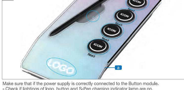
Make sure that if the power supply is correctly connected to the Button module.
