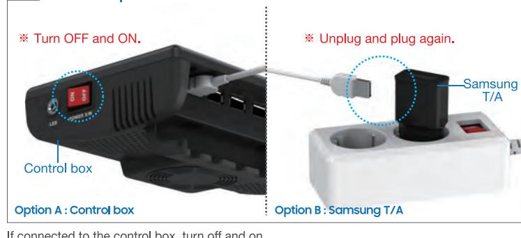
If connected to the control box, turn off and on.
