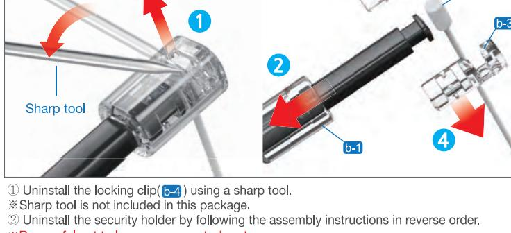
① Uninstall the locking clip (b-4) using a sharp tool.
