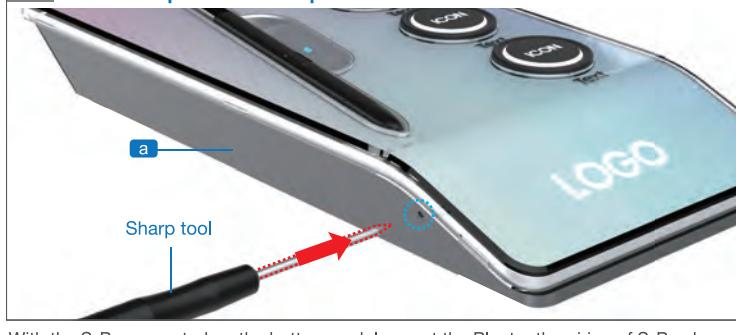
With the S-Pen mounted on the button module, reset the Bluetooth pairing of S-Pen by pressing the hole as shown in the figure above at the left side of the button module (a) for approximately 1 second using a sharp tool.
