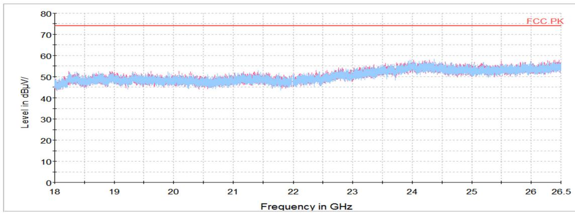
**Simultaneously – BLE(2402 MHz) + WPT(Charging)**
