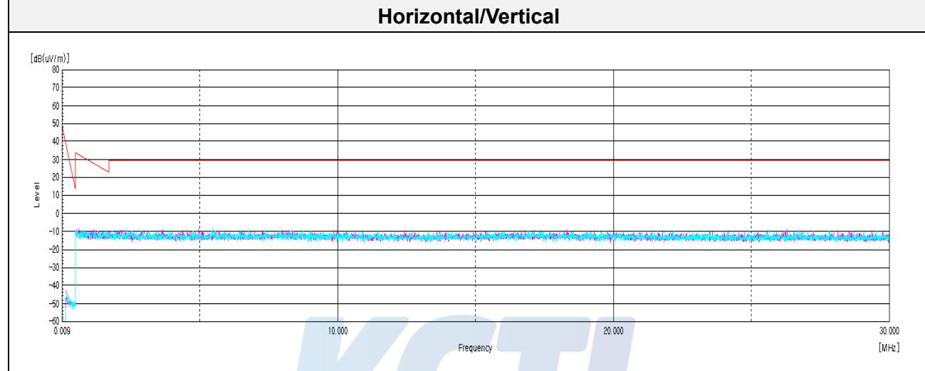
**Test results (Below 1 000 MHz) Worst case: BLE\_1 MBit/s(37 Bytes) Lowest frequency**
