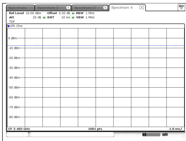
Note<sub>1</sub> : BLE (1MBits/s, Packet length 37) is a continuous transmission (duty cycle  $\geq 98\%$ )
