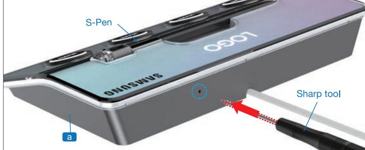
With the S-Pen mounted on the button module, reset the Bluetooth pairing of S-Pen by pressing the hole as shown in the figure above at the back of the button module (a) for approximately 1 second using a sharp tool.
