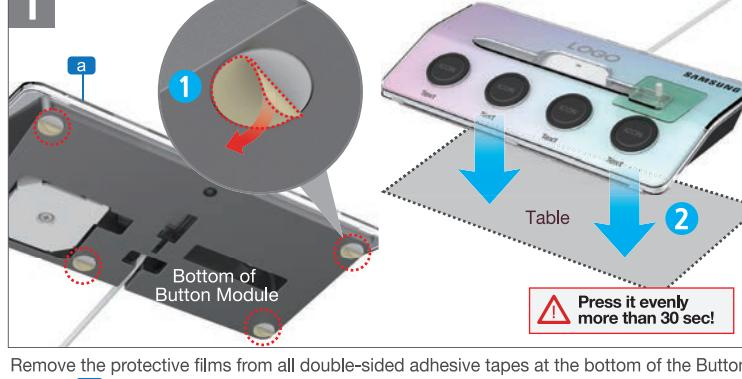
Remove the protective films from all double-sided adhesive tapes at the bottom of the Button module (a) and firmly attached the Button module on the table.
