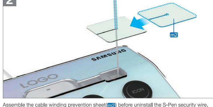
Assemble the cable winding prevention sheet (m2) before uninstall the S-Pen security wire.
