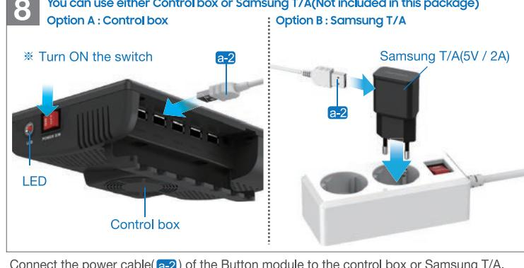
Connect the power cable (a-2) of the Button module to the control box or Samsung T/A.
