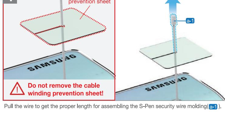
Pull the wire to get the proper length for assembling the S-Pen security wire molding (a-1).
