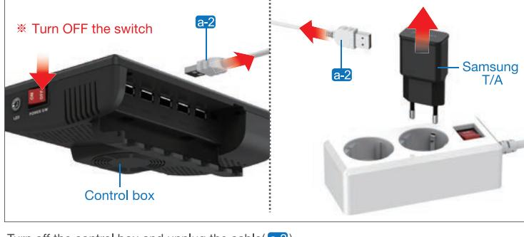
Turn off the control box and unplug the cable (a-2).
