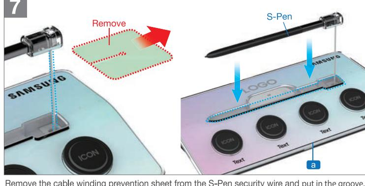
Remove the cable winding prevention sheet from the S-Pen security wire and put in the groove.
