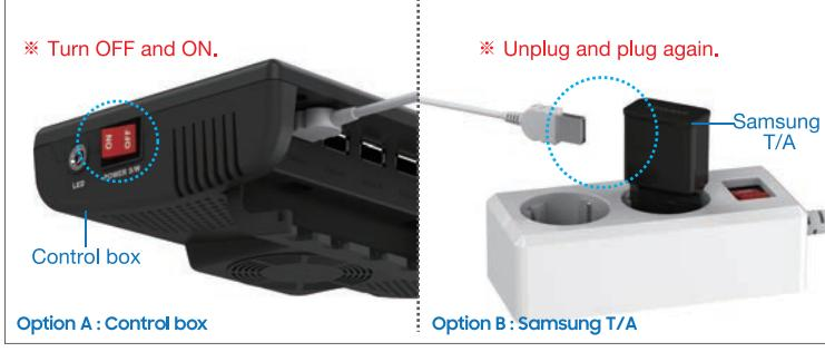
If connected to the control box, turn off and on. If connected to a Samsung T/A, unplug and plug again the button module cable.
