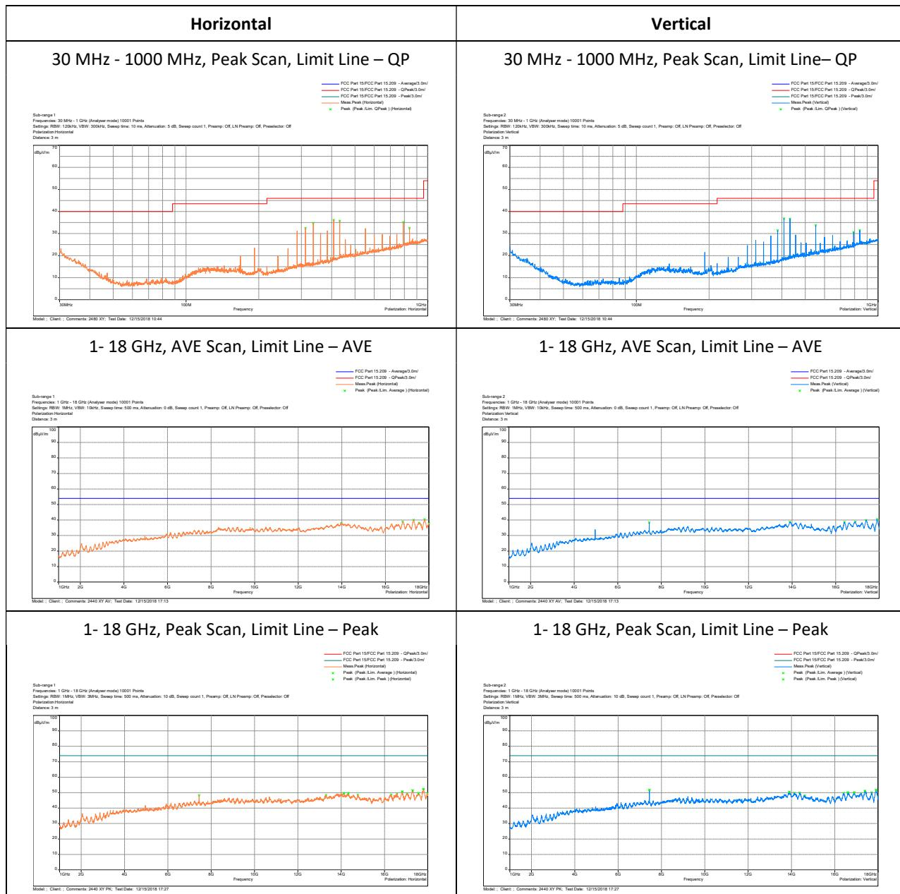
Note: Radiated spurious emissions measurements were performed from 30 MHz to 25 GHz.
