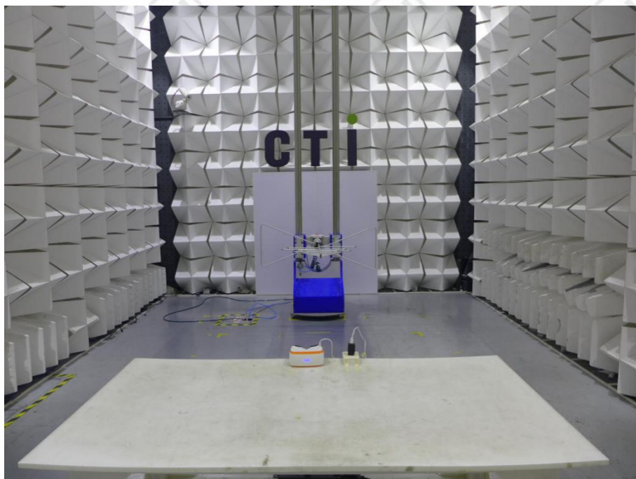
Radiated spurious emission Test Setup-1(Below 1GHz)
