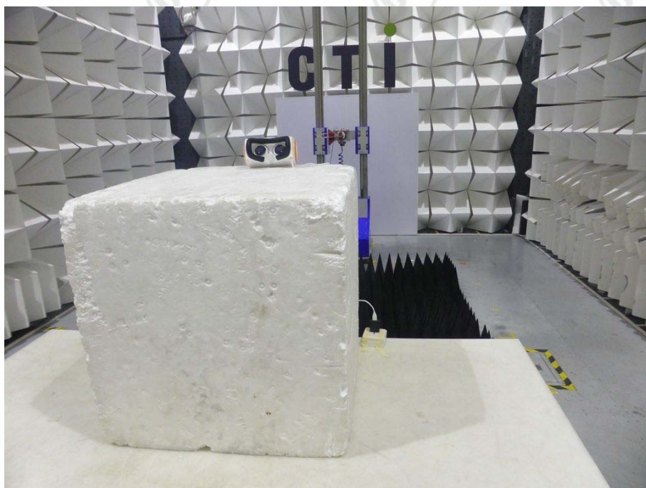
Radiated spurious emission Test Setup-2(Above 1GHz)
