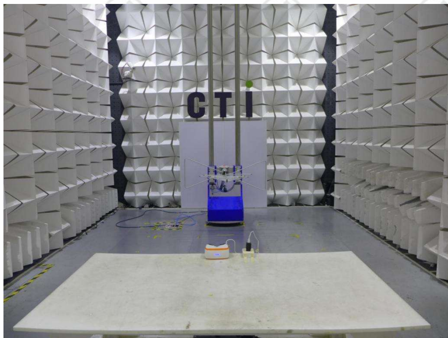
Radiated spurious emission Test Setup-1(Below 1GHz)
