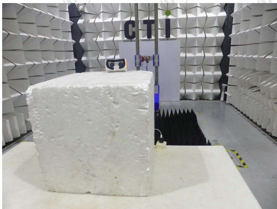
Radiated spurious emission Test Setup-2(Above 1GHz)
