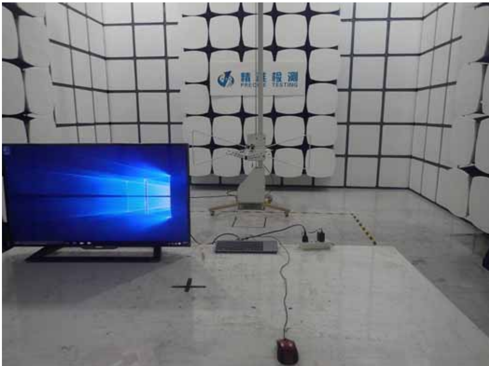
FCC RADIATED EMISSION TEST SETUP BELOW 1GHZ
