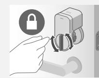
When the lock/unlock position is stored on Smart Lock, Smart Lock will start testing the unlock movement automatically.
