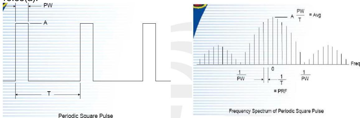
If using spectrum analyzer to measure pulse signal , it have to make sure the RBW use is at least  $2/PW$ .
