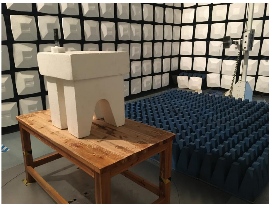
Test Setup For Radiated Emission (Above 1GHz)
