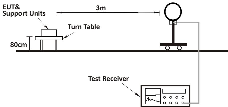
**For Radiated emission 30MHz to 1GHz:**
