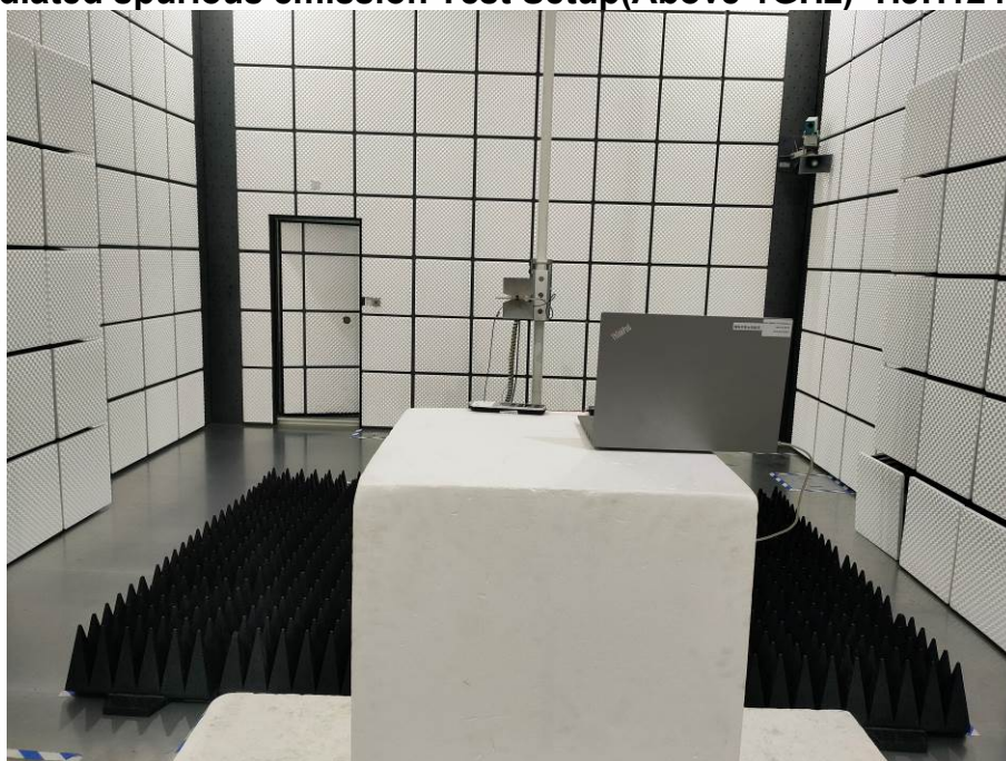
Radiated spurious emission Test Setup(Above 1GHz)- HJH124 Ble
