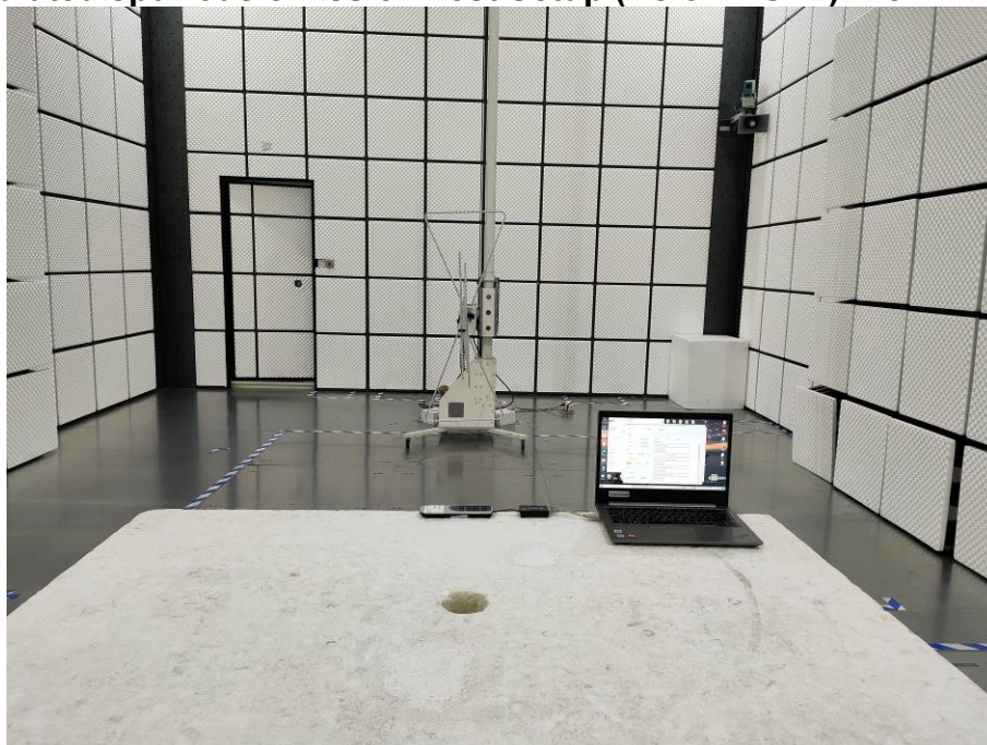
Radiated spurious emission Test Setup (Below 1GHz)- HJH124 Ble
