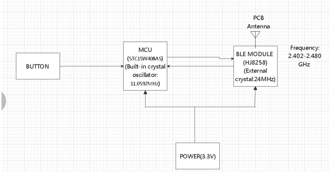
The HJH124 Ble remote control is mainly used for the control of household electric bed products to realize wireless control of the motor.
