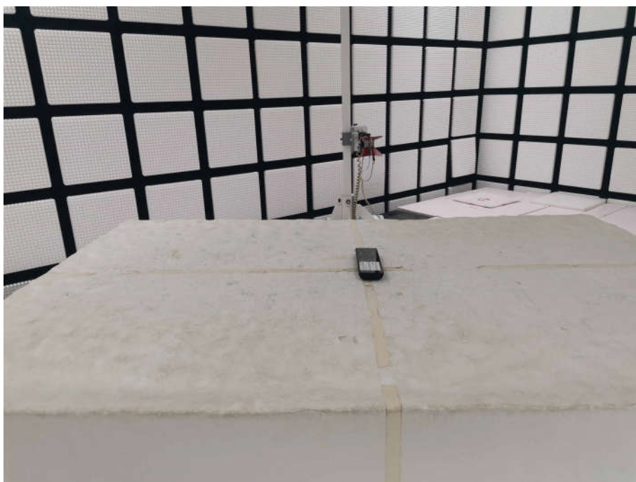
Radiated spurious emission Test Setup-2(Above 1GHz)
