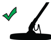
Correct search coil angle
