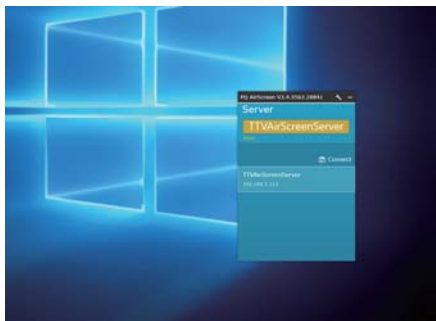
2.4 Tap "Connect" to start casting your laptop screen to your touch screen TV
