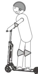
Step 4: Hold the handle, step on the pedal to keep balance, press accelerator to start.
