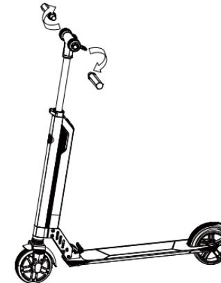
Step 4: You would install the handspike according to the direction in figure.
