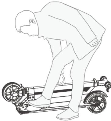
Step 1: Slam down foldable shield, when the axle separates from slot A completely, hold up the F0 body, then do the next steps.
