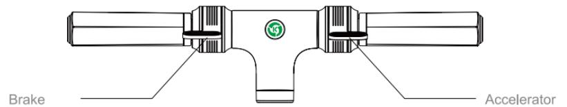
Brake: F0 use electronic brake. You press bigger range of brake crank, you will get bigger brake force. When you are in brake, you can't use accelerator.
