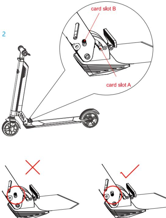
Step 2: Please keep axle snap into slot B utterly, then flip up the foldable shield to fit arc, otherwise your riding will be dangerous.
