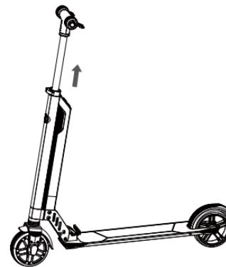
Step 3: Open "Fast locking device", set handle to appropriate height and fix it.
