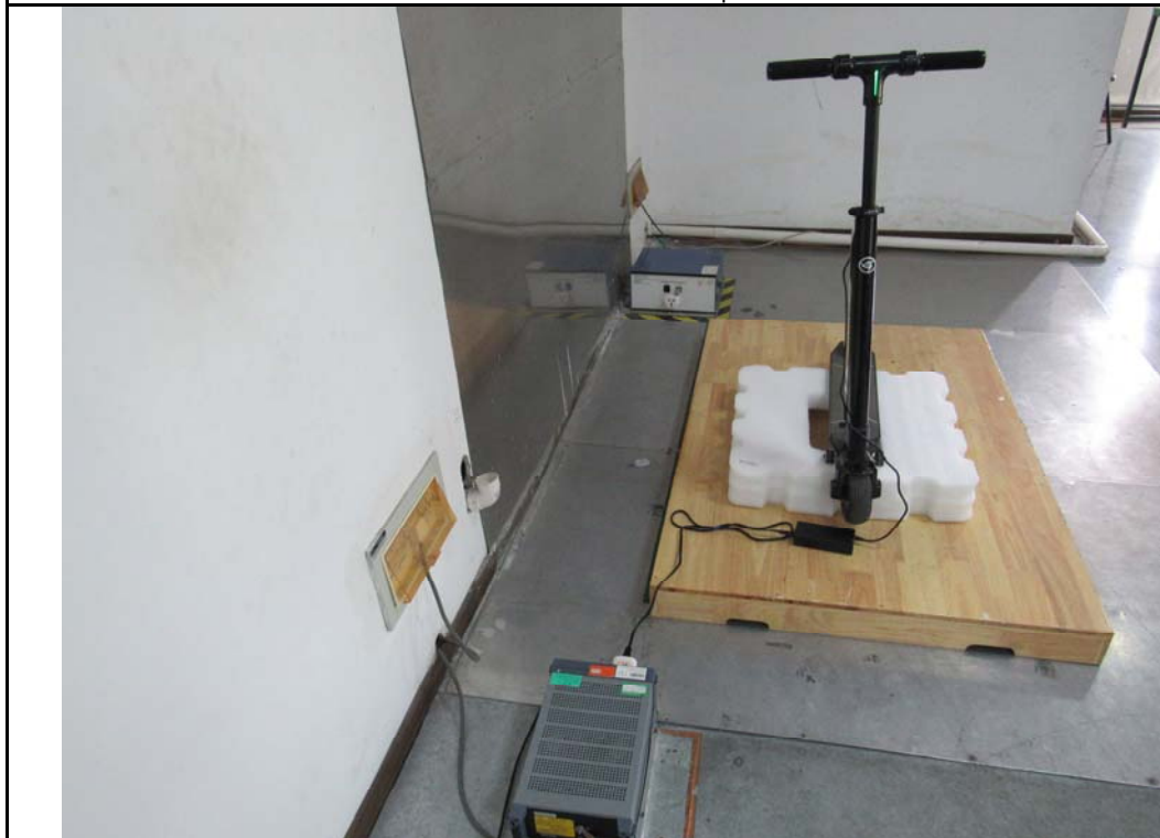
Conducted Emissions Test Setup Side View
