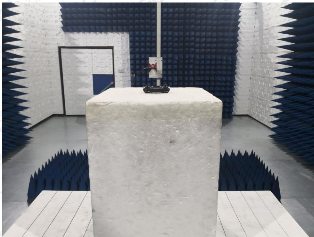
FCC RADIATED EMISSION TEST SETUP ABOVE 1GHZ
