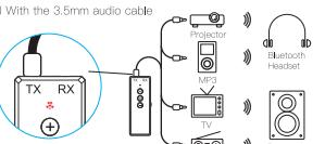
Plug one end of the 3.5mm audio cable into the audio interface (marked TX) on the transceiver, and the other end into the AUX interface on the TV or other equipment.
