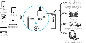
Plug the 3.5mm audio cable of the wired headset or wired speaker into the audio interface (marked RX) on the Bluetooth transceiver.
