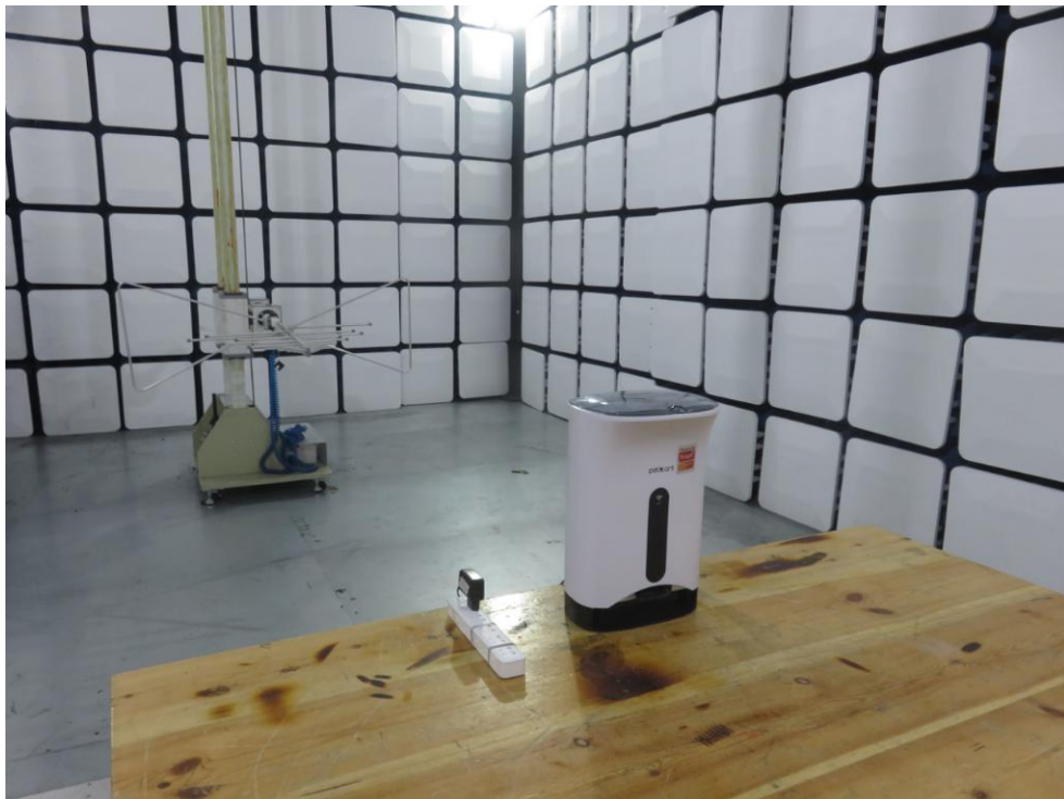
Photo of Radiation Emission Test
