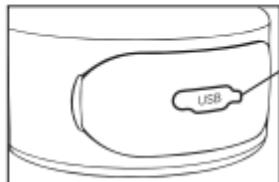
When the device is at low power, remove the plug and charge it using the micro USB cable.
