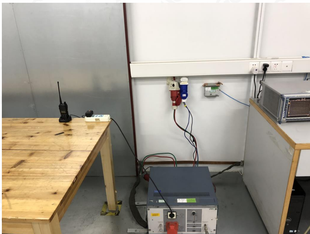
RADIATED EMISSION TEST SETUP-BELOW 1GHZ
