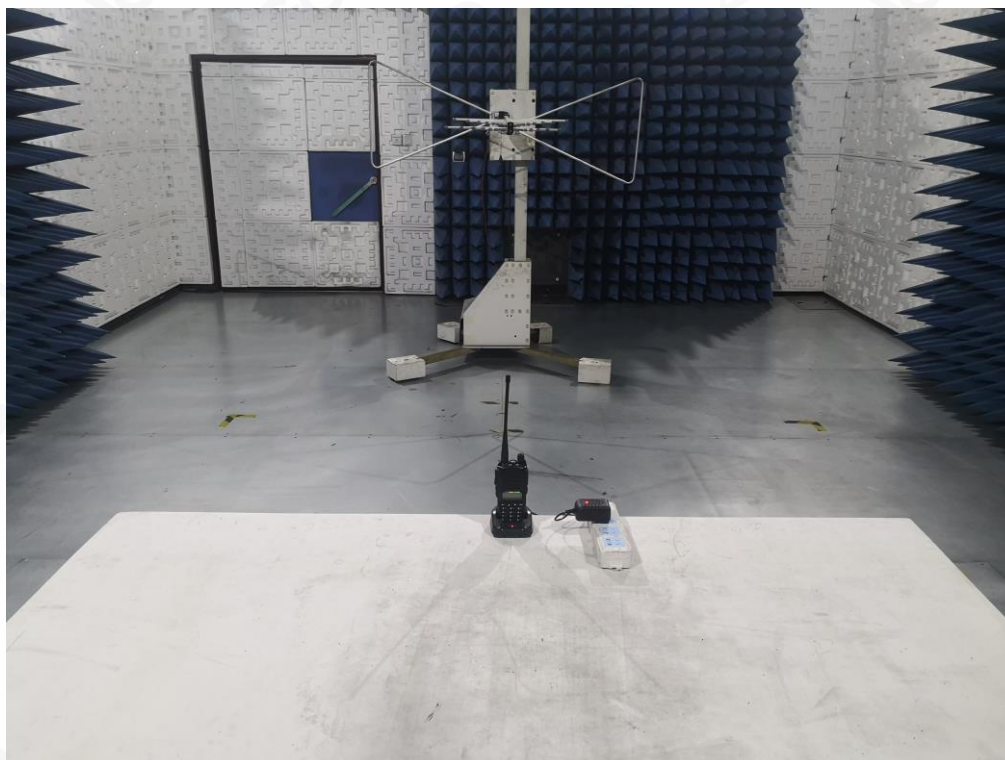
RADIATED EMISSION TEST SETUP-BELOW 1GHZ
