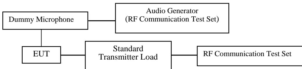
Setup Block Diagram for Audio Frequency filter:
