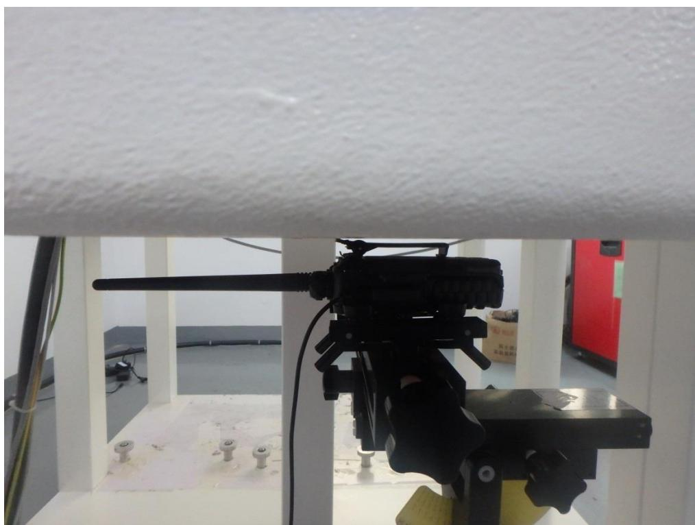
The thickness of EUT is 3.0 cm
