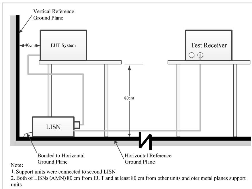
The measurement procedure of test setup is according with ANSI C63.4-2014. The related limit was specified in FCC Part 15.107 Class B limits.
