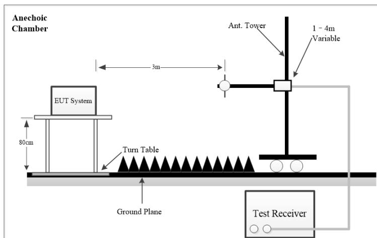
The radiated emission tests were performed in the 3 meters chamber test site, using the setup accordance with the ANSI C63.4-2014. The specification used was the FCC Part 15.109 Class B limits.
