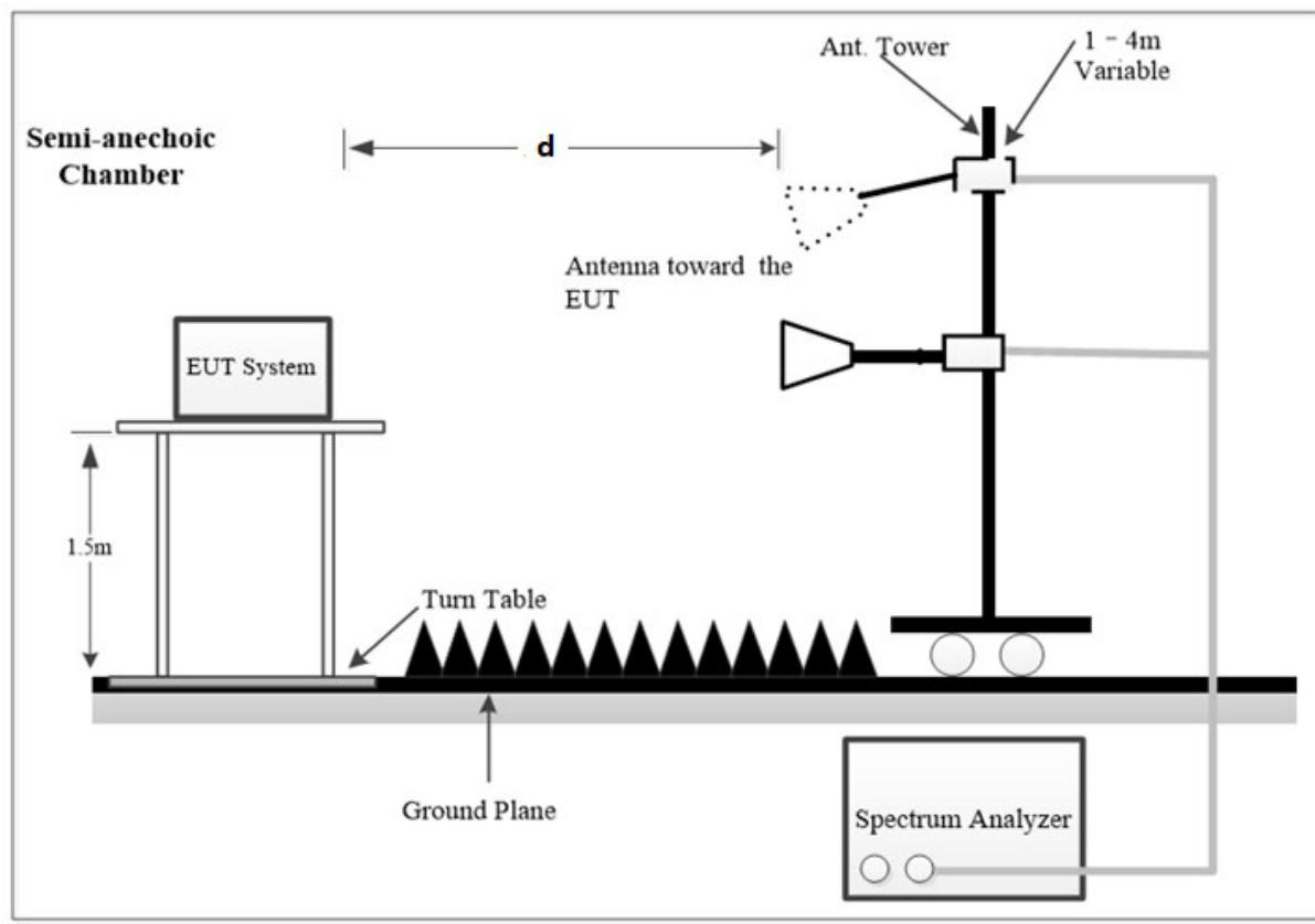
The radiated emission tests using the setup accordance with the ANSI C63.10-2013. The specification used was the FCC 15.209, and FCC 15.247 limits.
