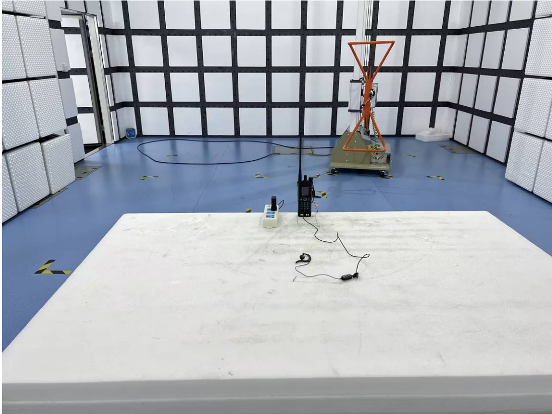
Radiation Emission_30MHz~1GHz - Rear View (Adapter Mode)
