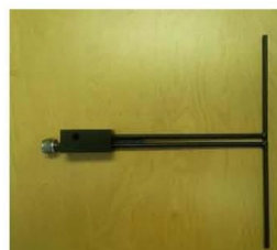
Figure 1 – MVG COMOSAR Validation Dipole
