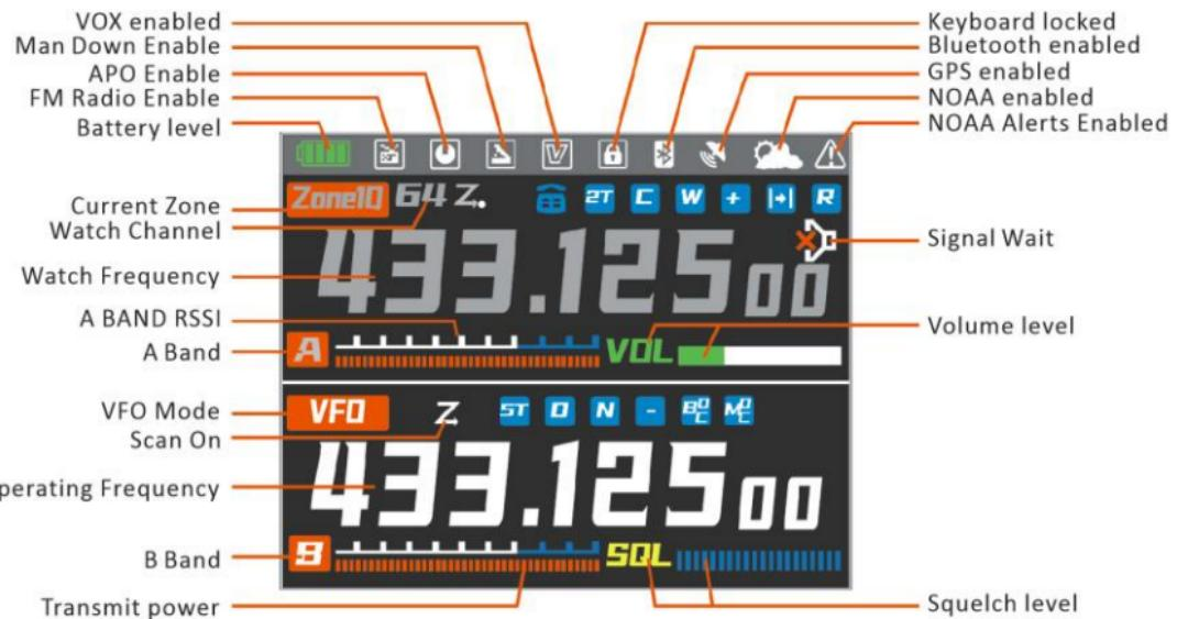
\*The highlighted band is the main channel (i.e., the working band) and the grayed-out band is the sub band (the watch band).
