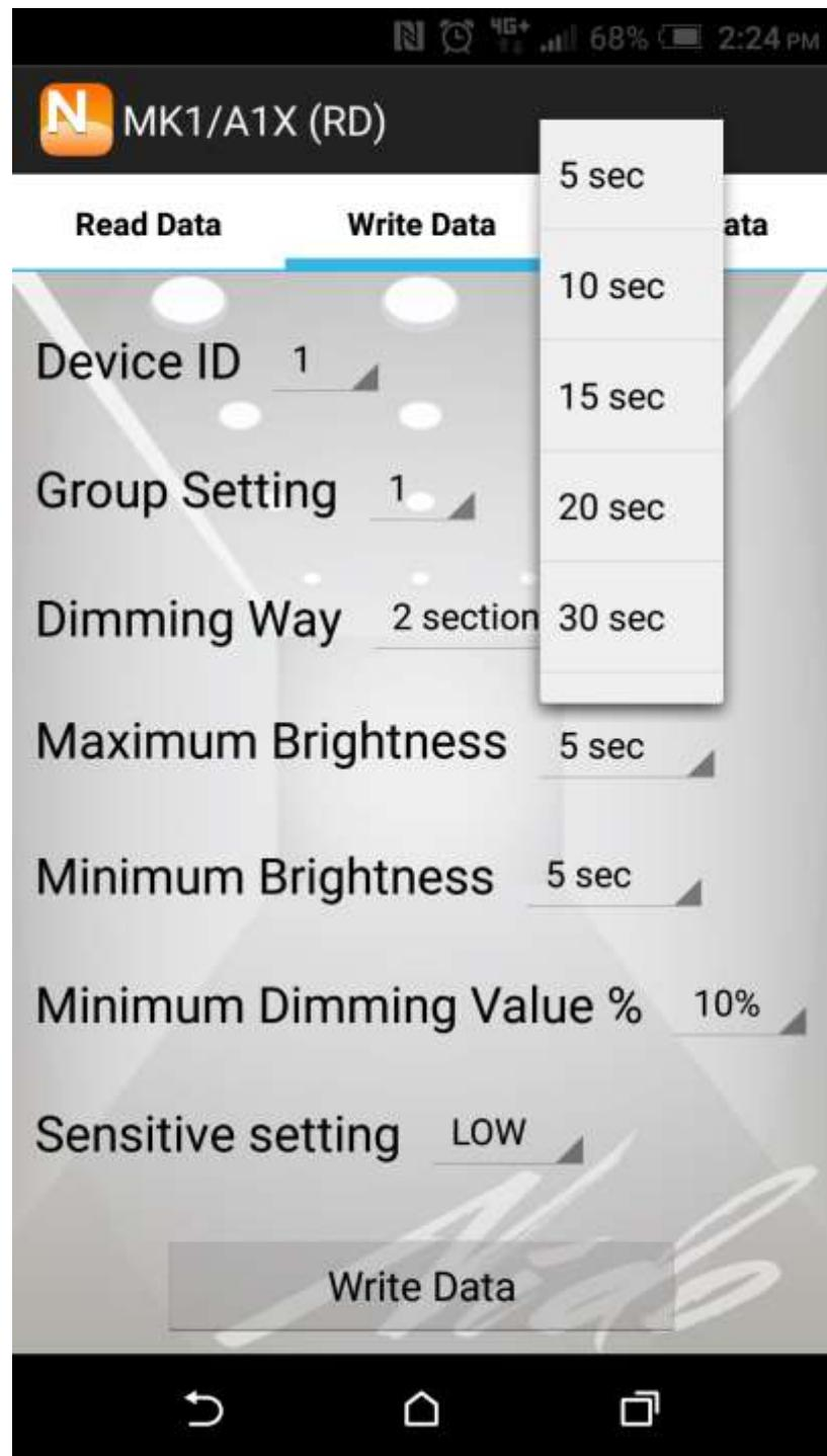
Minimum Brightness: in 3 sections dimming way, when a moving object has been detected by MK1, turn the lights up to 100% brightness. After the Maximum brightness mode, turn into minimum brightness mode, user can adjust the minimum brightness time as well (one hour top). After the time user sets, lights will turn off.
