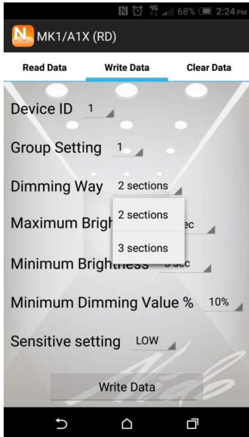
Maximum Brightness: In 2 sections/ 3 sections dimming way, when a moving object has been detected by MK1, turn the lights up to 100% brightness. User can adjust the Maximum brightness time. (one hour top)
