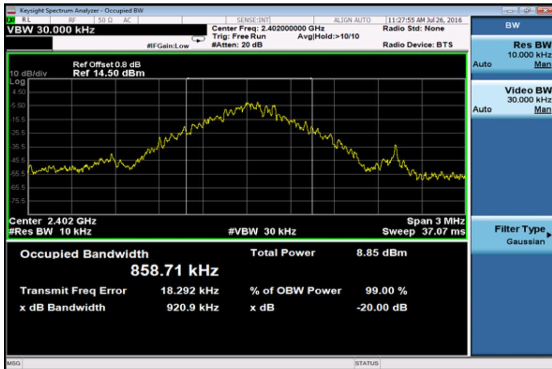
**20dB Bandwidth Test Data CH-Mid**
