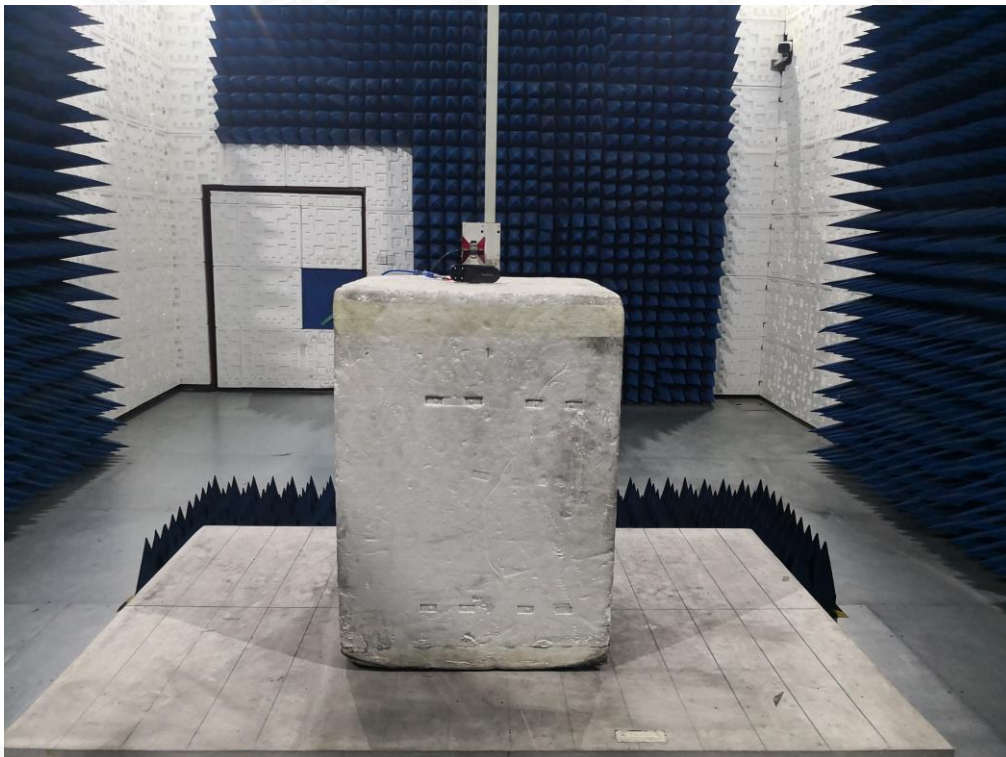
FCC RADIATED EMISSION TEST SETUP ABOVE 1GHZ
